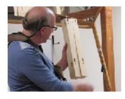
Stiles and rails were joined using half-through, stopped tenons. (see photographs). He uses a German mortise which is no longer made and for which the bits run \$200-\$300. He uses 3/8" square pegs into 3/8" round holes and bevels the leading ends to somewhat round. To make sure the subassemblies are flat he clamps them to a flat surface before pinning.
