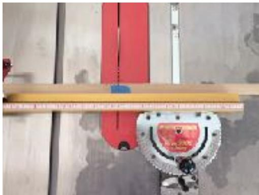
Without thinking, I turned on the saw and treated the miter gage as if it were a crosscut sled. Bang!!! The safety mechanism on the SawStop activated and here is what the blade and SawStop cartridge looked like.
