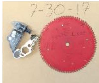
Nineteen teeth of an 80 tooth blade were damaged before the aluminum block stopped the rotating saw blade. The miter gage had a nick but is still functional.
