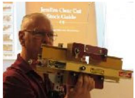
post further information with the AWA video. This jig has a built-in backer board, and built in micro-adjust. Tracy felt setup time is reasonable. Don't forget that after you add glue, the joint will be much tighter. The jig keeps your fingers away from the blade. Tracy likes this jig especially for making shop drawers from Baltic birch plywood. He says it is fast to use, fast to setup, and Tracy is very satisfied. Jerry Trujillo also endorses this product.
