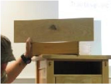
Glen said that after six years, this cabinet has had some shrinkage and expansion and he felt the grooves for the inset side panels weren't deep enough. He would have done some things differently. He said he'd make the groove deeper and probably use space balls next time. Bottom joint
