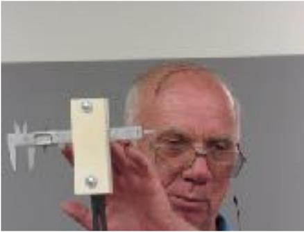
**Jack Henning** was the second speaker. He shared two clever, simple jigs he has made. The first jig checks that the saw blade is parallel to the table saw mitre slot, using an inexpensive (nondigital) caliper. The second was a thin rip guide.
