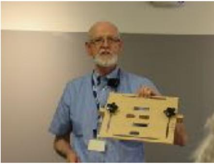
**Ben Blackwell** presented his 1/4" melamine (or MDF) based mortising jig. Ben's design differed from the other two designs. For a desired mortise length and width, there is a specific combination of router bit diameter, guide bushing (with an outside and inside diameter) and slot geometry in the melamine base to
