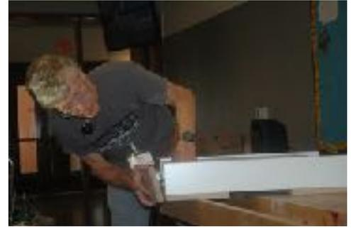
The 3-ply bamboo plywood used in the cabinets provides a warm color without staining and an interesting exposed edge effect. The bamboo machines the same as wood (similar to walnut). Controlled humidity (around 30%) is required to prevent checking. Other forms of the bamboo plywood are available. The video from the presentation describes the process of making the plywood (starting at about 64 minutes).
