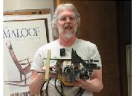
Gale showed an inventive circle cutting jig with 3/32” holes (sized to 6p nail) every 1/2” and a sliding baseplate adjustment that gives him unlimited circle diameter cutting capability within the minimum and maximum parameters of the jig.
